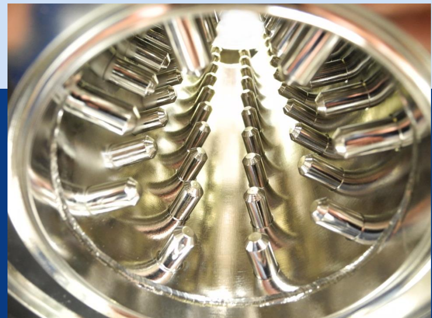
Round pin shape mixer design. Hygienic design
